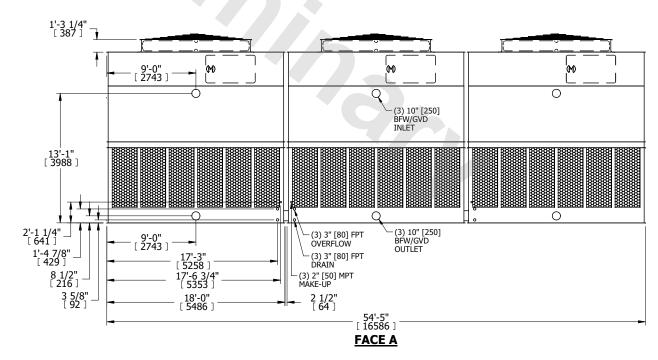
DRAWN BY: KDS NO. OF SHIPPING SECTIONS **SHIPPING** OPERATING HEAVIEST SECTION 38820 lbs+ [17610] kg+ 66630 lbs+ [30225] kg+ 8760 lbs+ [3975] kg+ WEIGHT WEIGHT WEIGHT
