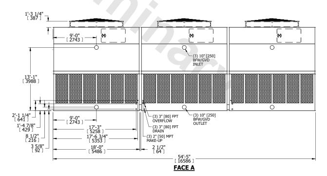
DRAWN BY: KDS NO. OF SHIPPING SECTIONS **SHIPPING** OPERATING HEAVIEST SECTION 39150 lbs+ [17760] kg+ 66960 lbs+ [30375] kg+ 8870 lbs+ [4025] kg+ WEIGHT WEIGHT WEIGHT
