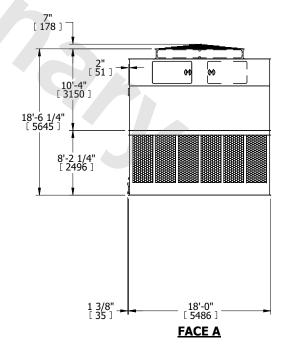
DRAWN BY: KDS NO. OF SHIPPING SECTIONS **SHIPPING OPERATING** HEAVIEST SECTION 26500 lbs+ [12025] kg+ 45040 lbs+ [20430] kg+ 8870 lbs+ [4025] kg+ WEIGHT WEIGHT WEIGHT
