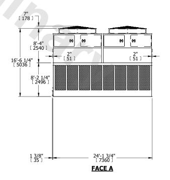
SHIPPING WEIGHT 31780 lbs+ [14420] kg+ OPERATING WEIGHT 56100 lbs+ [25450] kg+ HEAVIEST SECTION WEIGHT 5790 lbs+ [2630] kg+ NO. OF SHIPPING SECTIONS 6 DRAWN BY: JLG
