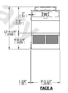
SHIPPING WEIGHT 7960 lbs+ [3615] kg+ OPERATING WEIGHT 12800 lbs+ [5810] kg+ HEAVIEST SECTION WEIGHT 2640 lbs+ [1200] kg+ NO. OF SHIPPING SECTIONS 4 DRAWN BY: JLG
