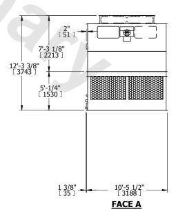
SHIPPING WEIGHT 9840 lbs+ [4465] kg+ OPERATING WEIGHT 16440 lbs+ [7460] kg+ HEAVIEST SECTION WEIGHT 3200 lbs+ [1455] kg+ NO. OF SHIPPING SECTIONS 4 DRAWN BY: JLG
