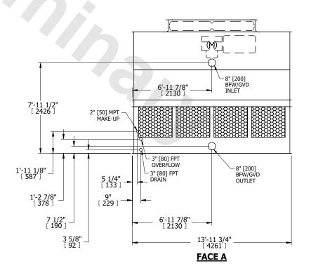
SHIPPING WEIGHT 5730 lbs+ [2600] kg+ OPERATING WEIGHT 10240 lbs+ [4645] kg+ HEAVIEST SECTION WEIGHT 3680 lbs+ [1670] kg+ NO. OF SHIPPING SECTIONS 2 DRAWN BY: JLG
