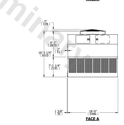
DRAWN BY: JLG NO. OF SHIPPING SECTIONS **SHIPPING** OPERATING HEAVIEST SECTION 20620 lbs+ [9355] kg+ 35820 lbs+ [16250] kg+ 6400 lbs+ [2905] kg+ WEIGHT WEIGHT WEIGHT
