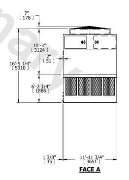
SHIPPING WEIGHT 15240 lbs+ [6915] kg+ OPERATING WEIGHT 25160 lbs+ [11415] kg+ HEAVIEST SECTION WEIGHT 5170 lbs+ [2350] kg+ NO. OF SHIPPING SECTIONS 4 DRAWN BY: JLG
