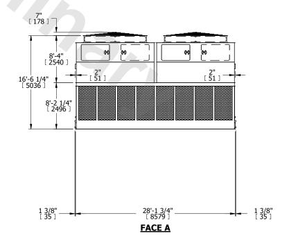
**SHIPPING OPERATING** HEAVIEST SECTION 35580 lbs+ [16140] kg+ 64480 lbs+ [29250] kg+ WEIGHT WEIGHT WEIGHT
