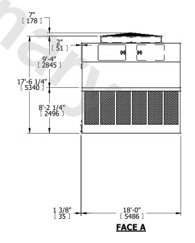
DRAWN BY: KDS NO. OF SHIPPING SECTIONS **SHIPPING** OPERATING HEAVIEST SECTION 24800 lbs+ [11250] kg+ 43340 lbs+ [19660] kg+ 8020 lbs+ [3640] kg+ WEIGHT WEIGHT WEIGHT
