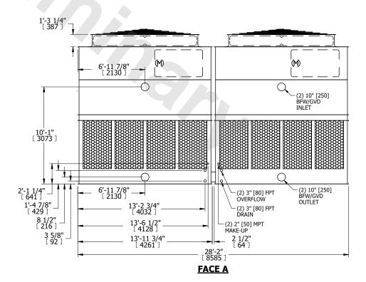
DRAWN BY: KDS NO. OF SHIPPING SECTIONS **SHIPPING** OPERATING HEAVIEST SECTION 17200 lbs+ [7805] kg+ 5550 lbs+ [2520] kg+ 31860 lbs+ [14455] kg+ WEIGHT WEIGHT WEIGHT
