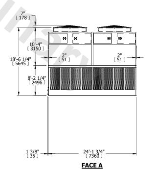
SHIPPING WEIGHT 35900 lbs+ [16285] kg+ OPERATING WEIGHT 60220 lbs+ [27320] kg+ HEAVIEST SECTION WEIGHT 6080 lbs+ [2760] kg+ NO. OF SHIPPING SECTIONS 6 DRAWN BY: JLG
