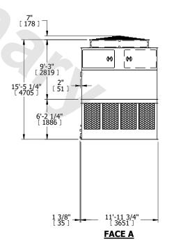
SHIPPING WEIGHT 14500 lbs+ [6580] kg+ OPERATING WEIGHT 24420 lbs+ [11080] kg+ HEAVIEST SECTION WEIGHT 4800 lbs+ [2180] kg+ NO. OF SHIPPING SECTIONS 4 DRAWN BY: KDS
