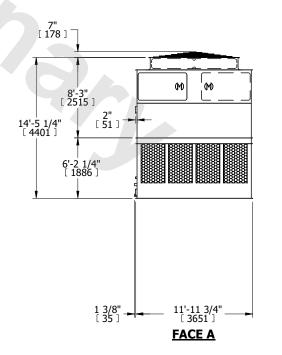
SHIPPING WEIGHT 13440 lbs+ [6100] kg+ OPERATING WEIGHT 23360 lbs+ [10600] kg+ HEAVIEST SECTION WEIGHT 4270 lbs+ [1940] kg+ NO. OF SHIPPING SECTIONS 4 DRAWN BY: JLG
