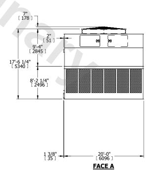
SHIPPING WEIGHT 25960 lbs+ [11780] kg+ OPERATING WEIGHT 46760 lbs+ [21210] kg+ HEAVIEST SECTION WEIGHT 8360 lbs+ [3795] kg+ NO. OF SHIPPING SECTIONS 4 DRAWN BY: BLL
