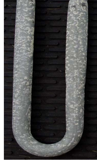
White rusted coil
