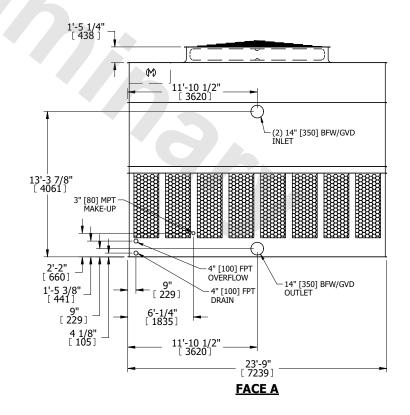
DRAWN BY: TAM NO. OF SHIPPING SECTIONS **SHIPPING** OPERATING HEAVIEST SECTION 19940 lbs+ [9045] kg+ 14100 lbs+ [6400] kg+ 36220 lbs+ [16430] kg+ WEIGHT WEIGHT WEIGHT
