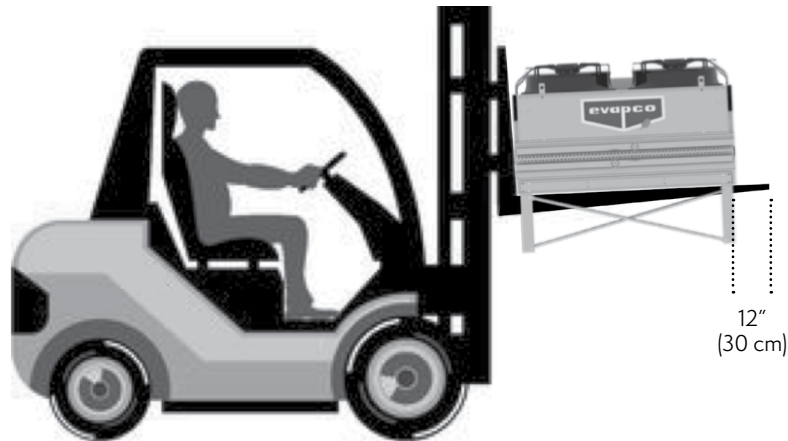
Figure 4 – Flat Coil Unit Forklift Lifting Requirements
