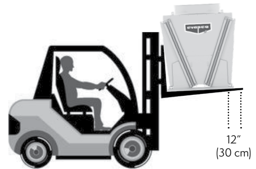
Figure 12 – V-Coil Unit Forklift Lifting Requirements
