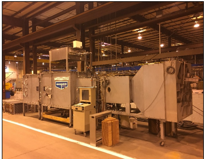
Figure 5: Evapco Adiabatic Pad Test Chamber
