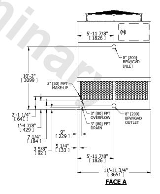
SHIPPING WEIGHT 8630 lbs+ [3915] kg+ OPERATING WEIGHT 14840 lbs+ [6735] kg+ HEAVIEST SECTION WEIGHT 6230 lbs+ [2830] kg+ NO. OF SHIPPING SECTIONS 2 DRAWN BY: KDS
