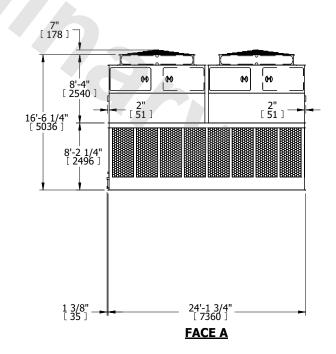
SHIPPING WEIGHT 32380 lbs+ [14690] kg+ OPERATING WEIGHT 56700 lbs+ [25720] kg+ HEAVIEST SECTION S790 lbs+ [2630] kg+
