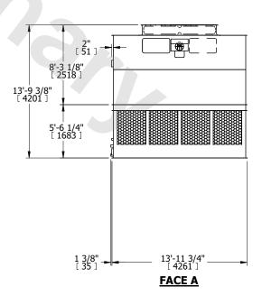
DRAWN BY: KDS NO. OF SHIPPING SECTIONS **SHIPPING** OPERATING HEAVIEST SECTION 12800 lbs+ [5810] kg+ 4260 lbs+ [1935] kg+ 21820 lbs+ [9900] kg+ WEIGHT WEIGHT WEIGHT
