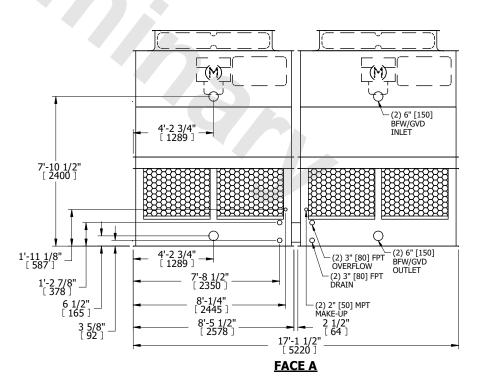
SHIPPING WEIGHT 7140 lbs+ [3240] kg+ OPERATING WEIGHT 11980 lbs+ [5435] kg+ HEAVIEST SECTION WEIGHT 2260 lbs+ [1030] kg+ NO. OF SHIPPING SECTIONS 4 DRAWN BY: JLG
