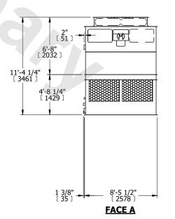
DRAWN BY: JLG NO. OF SHIPPING SECTIONS **SHIPPING** OPERATING HEAVIEST SECTION 7380 lbs+ [3350] kg+ 12220 lbs+ [5545] kg+ 2350 lbs+ [1070] kg+ WEIGHT WEIGHT WEIGHT
