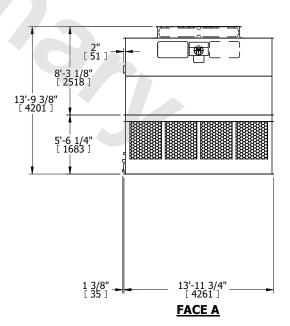
DRAWN BY: KDS NO. OF SHIPPING SECTIONS **SHIPPING** OPERATING HEAVIEST SECTION 12760 lbs+ [5790] kg+ 4240 lbs+ [1925] kg+ 21780 lbs+ [9880] kg+ WEIGHT WEIGHT WEIGHT
