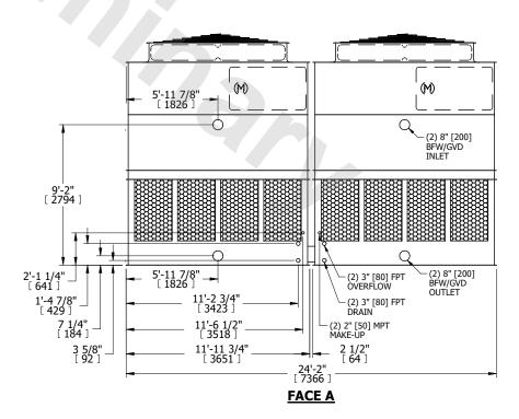
SHIPPING WEIGHT 15480 lbs+ [7025] kg+ OPERATING WEIGHT 27900 lbs+ [12660] kg+ HEAVIEST SECTION WEIGHT 5200 lbs+ [2360] kg+ NO. OF SHIPPING SECTIONS 4 DRAWN BY: KDS
