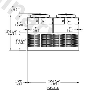
SHIPPING WEIGHT 31980 lbs+ [14510] kg+ OPERATING WEIGHT 56300 lbs+ [25540] kg+ HEAVIEST SECTION WEIGHT 5790 lbs+ [2630] kg+ NO. OF SHIPPING SECTIONS 6 DRAWN BY: JLG
