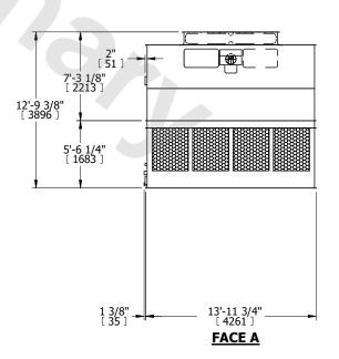
SHIPPING WEIGHT 11940 lbs+ [5420] kg+ OPERATING WEIGHT 20960 lbs+ [9510] kg+ HEAVIEST SECTION WEIGHT 3830 lbs+ [1740] kg+ NO. OF SHIPPING SECTIONS 4 DRAWN BY: KDS
