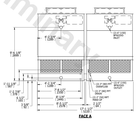
SHIPPING WEIGHT 7160 lbs+ [3250] kg+ OPERATING WEIGHT 11240 lbs+ [5100] kg+ HEAVIEST SECTION WEIGHT 2430 lbs+ [1105] kg+ NO. OF SHIPPING SECTIONS 4 DRAWN BY: JLG
