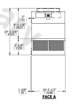
DRAWN BY: KDS NO. OF SHIPPING SECTIONS **SHIPPING** OPERATING HEAVIEST SECTION 10900 lbs+ [4945] kg+ 17500 lbs+ [7940] kg+ 3730 lbs+ [1695] kg+ WEIGHT WEIGHT WEIGHT
