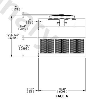
SHIPPING WEIGHT 25440 lbs+ [11540] kg+ OPERATING WEIGHT 46240 lbs+ [20975] kg+ HEAVIEST SECTION WEIGHT 8100 lbs+ [3675] kg+ NO. OF SHIPPING SECTIONS WEIGHT
