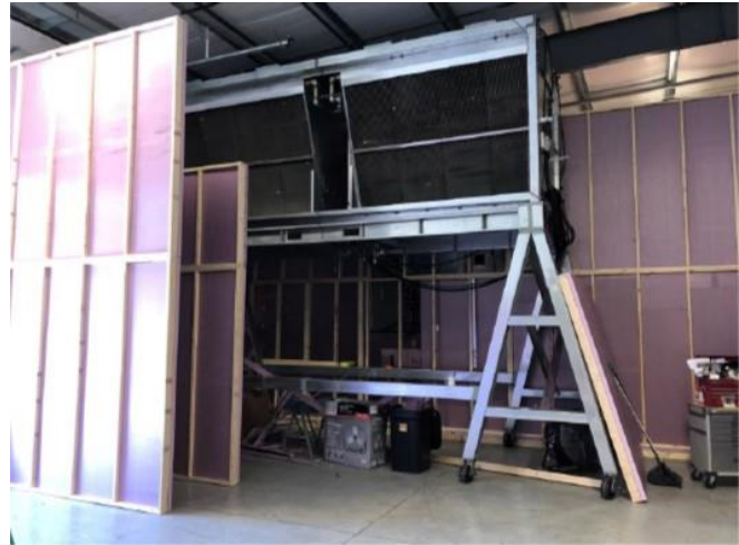
Figure 4: Condenser Installation in Low Ambient Test Chamber
