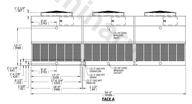
SHIPPING WEIGHT 37860 lbs+ [17175] kg+ OPERATING WEIGHT 65670 lbs+ [29790] kg+ HEAVIEST SECTION WEIGHT 8440 lbs+ [3830] kg+ NO. OF SHIPPING SECTIONS 6 DRAWN BY: KDS
