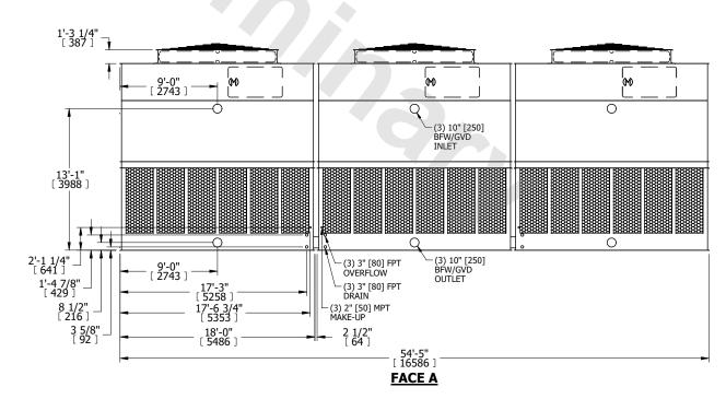
SHIPPING WEIGHT 38640 lbs+ [17530] kg+ OPERATING WEIGHT 66450 lbs+ [30145] kg+ HEAVIEST SECTION WEIGHT 8700 lbs+ [3950] kg+ NO. OF SHIPPING SECTIONS 6 DRAWN BY: KDS
