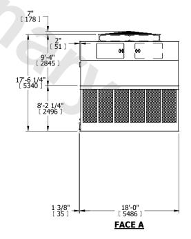
SHIPPING WEIGHT 24160 lbs+ [10960] kg+ OPERATING WEIGHT 42700 lbs+ [19370] kg+ HEAVIEST SECTION WEIGHT 7700 lbs+ [3495] kg+ NO. OF SHIPPING SECTIONS 4 DRAWN BY: KDS
