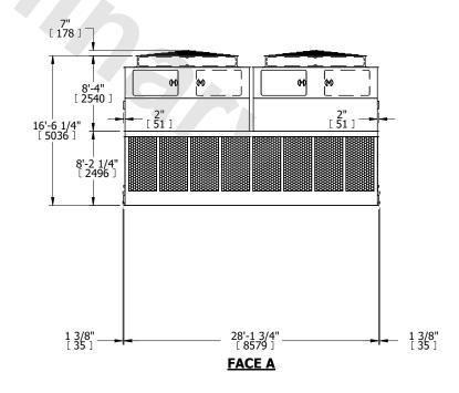
SHIPPING WEIGHT 35300 lbs+ [16015] kg+ OPERATING WEIGHT 64200 lbs+ [29125] kg+ HEAVIEST SECTION WEIGHT 6550 lbs+ [2975] kg+ NO. OF SHIPPING SECTIONS 6 DRAWN BY: JLG
