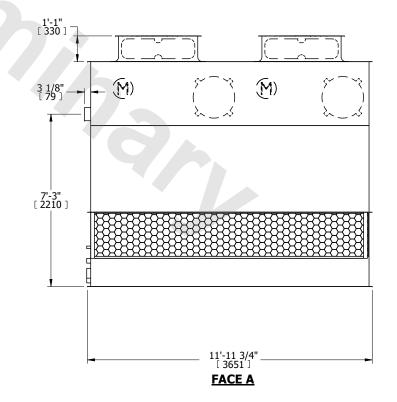
SHIPPING WEIGHT 2770 lbs+ [1260] kg+ OPERATING WEIGHT 4890 lbs+ [2220] kg+ HEAVIEST SECTION WEIGHT 2010 lbs+ [915] kg+ NO. OF SHIPPING SECTIONS 2 DRAWN BY: KWC
