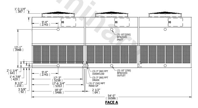
SHIPPING WEIGHT 37530 lbs+ [17025] kg+ OPERATING WEIGHT 65340 lbs+ [29640] kg+ HEAVIEST SECTION WEIGHT 8330 lbs+ [3780] kg+ NO. OF SHIPPING SECTIONS 6 DRAWN BY: KDS
