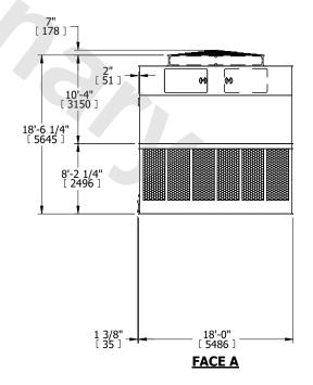
SHIPPING WEIGHT 25420 lbs+ [11535] kg+ OPERATING WEIGHT 43960 lbs+ [19940] kg+ HEAVIEST SECTION WEIGHT 8330 lbs+ [3780] kg+ NO. OF SHIPPING SECTIONS 4 DRAWN BY: KDS
