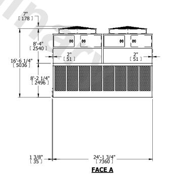
SHIPPING WEIGHT 31020 lbs+ [14075] kg+ OPERATING WEIGHT 55340 lbs+ [25105] kg+ HEAVIEST SECTION WEIGHT 5790 lbs+ [2630] kg+ NO. OF SHIPPING SECTIONS 6 DRAWN BY: JLG
