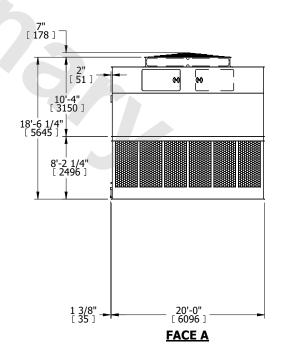
DRAWN BY: KDS NO. OF SHIPPING SECTIONS **SHIPPING** OPERATING HEAVIEST SECTION 27020 lbs+ [12260] kg+ 8890 lbs+ [4035] kg+ 47820 lbs+ [21695] kg+ WEIGHT WEIGHT WEIGHT
