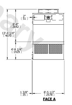
SHIPPING WEIGHT 7520 lbs+ [3415] kg+ OPERATING WEIGHT 11600 lbs+ [5265] kg+ HEAVIEST SECTION 2570 lbs+ [1170] kg+
