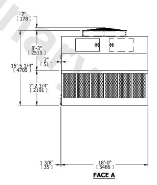
SHIPPING WEIGHT 19240 lbs+ [8730] kg+ OPERATING WEIGHT 34440 lbs+ [15625] kg+ HEAVIEST SECTION WEIGHT 5710 lbs+ [2595] kg+ NO. OF SHIPPING SECTIONS 4 DRAWN BY: KDS
