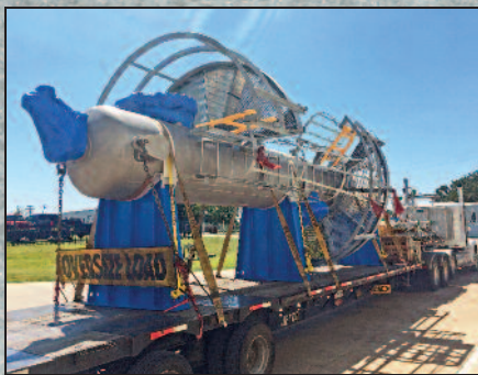
42" ID x 242" SM/SM Stainless Steel CO2 Water Wash Column with Ladders and Platforms
