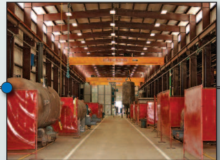
Three Manufacturing Bays, Twenty-Nine Vessel Welding Stations and Ten Overhead Cranes with Hoist Capacity of 200,000 lbs.
