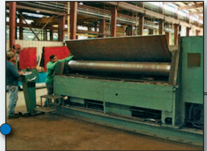
Plate Bending With Expanded Capacity to Roll Up to 10 Foot Wide x 1.5" Thick Steel Shells in 30" to 156" Diameters
