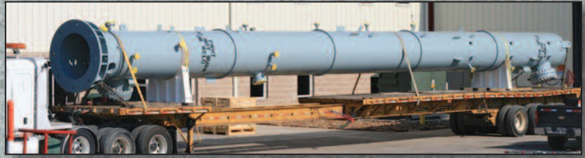
48" ID x 936" SM/SM Contactor Tower Ready for Shipment
