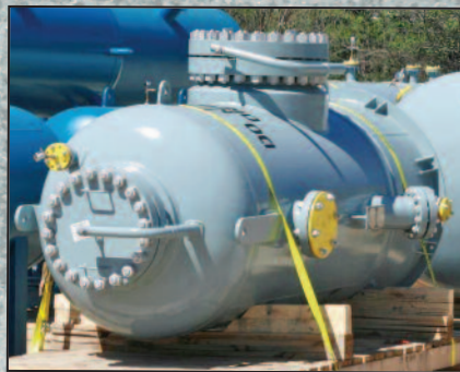
54" ID x 84" SM/SM Mercury Guard Bed & Scrubber
