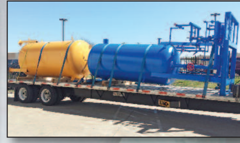
Pump Recirculator Package and High Pressure Receiver
