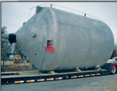
180" Diameter Stainless Steel Cone Head Recirculator
