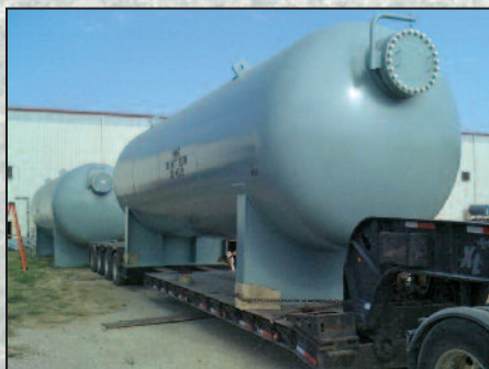
120" OD x 600" SM/SM Mixed Refrigerant Surge Drum
