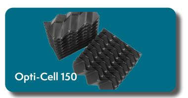
OC-150 drift eliminators remove water droplets from the air stream with minimal pressure loss in both counter-flow and cross-flow cooling towers. Made from rigid PVC, they consist of alternating corrugated and sine wave sheets bonded between 1.5" spacer sheets.
