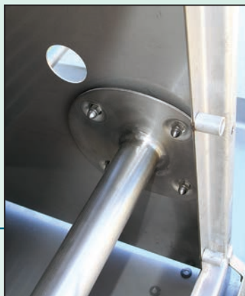
Shaft motor support with "spacer" for complete cleaning between the end bracket and the side panel.
